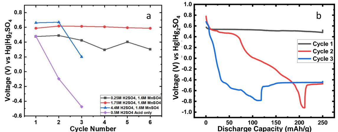
**Figure 3.** (a) Effect of acid concentration and Mn<sup>2+</sup> on average discharge potential (b) Effect of absence of Mn<sup>2+</sup> ions in acid only electrolyte on the reversibility of the cathode reaction
