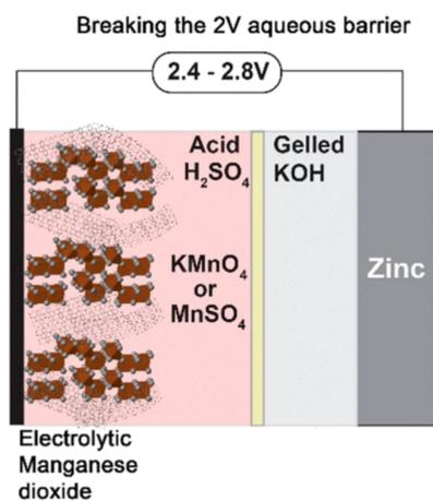
**Figure 1.** Schematic Diagram of the Dual Electrolyte High Voltage Zn|MnO<sub>2</sub> Battery
