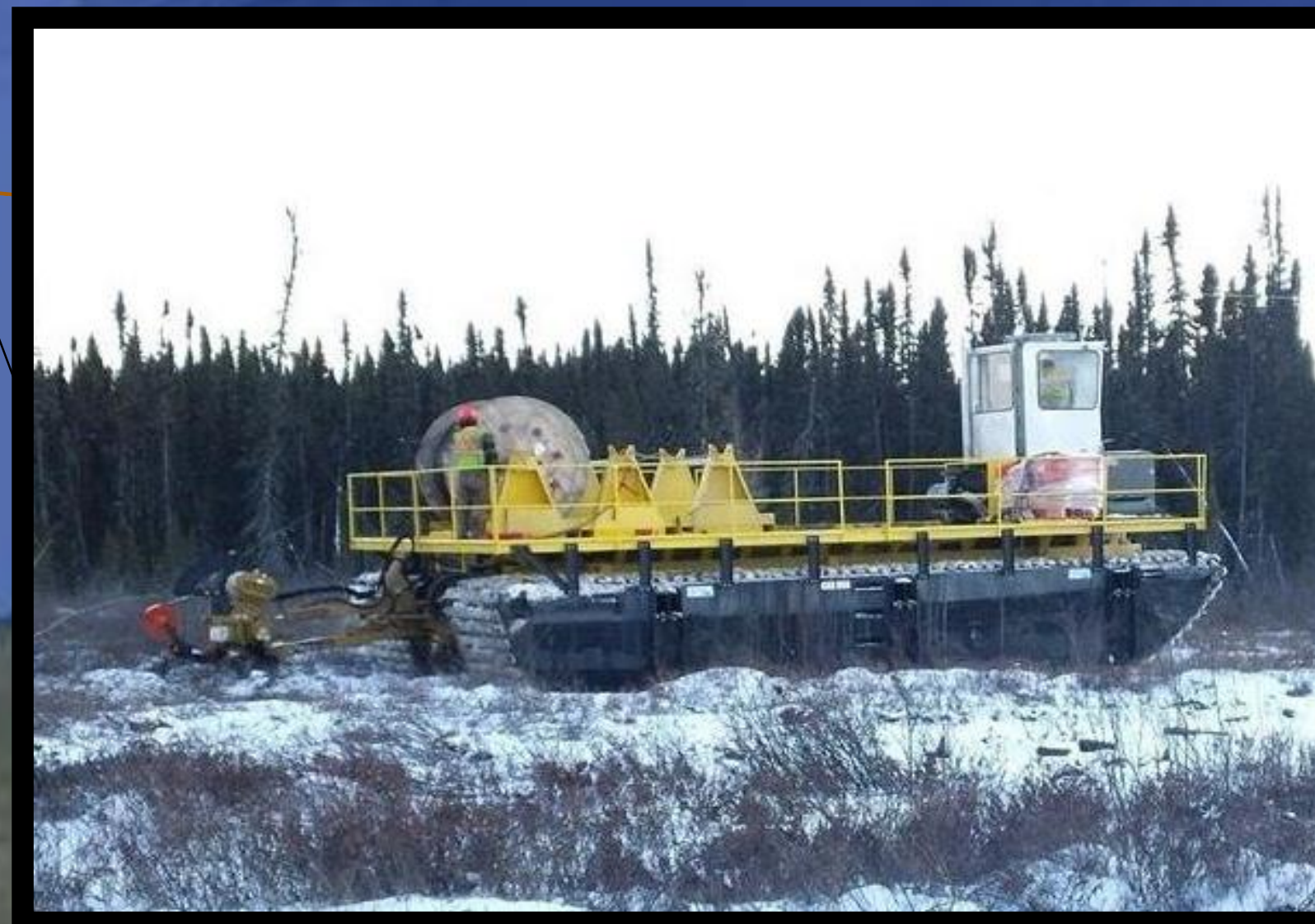
Fig. 2. Wetland Equipment Company amphibious vehicle used to lay cable on soft in wetlands and boggy tundra. Source: https://wetlandequipment.com/photo-gallery/5 , accessed 2020-09-14
